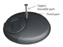
After emptying the refuse from the lifting container, close the lifting container's bottom part by lifting the upper part of the mushroom. Make sure the bottom is closed tightly before the lifting container is returned to the well. Check that there is no debris on the bottom of the well that will prevent the lifting container from settleing on the well correctly. When the lifting container is returned to the Molok® container, the upper part of the mushroom can be released down
